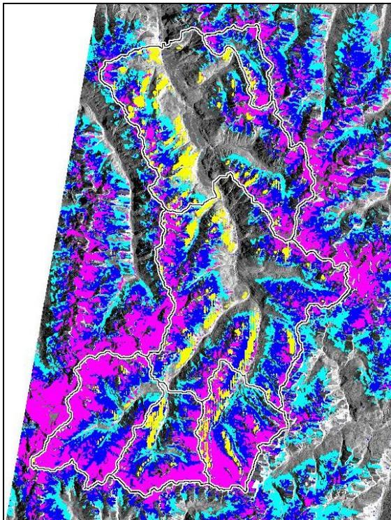
Fig. 10: Multitemporal snow map from ASAR IS-6, images, track 308 superimposed to a geocoded multitemporal amplitude image. Decrease of snow area from 4 May 2004 to 8 June 2004 (cyan), from 8 June 2004 to 13 July 2004 (blue), remaining snow extent on 13 July 2004 (magenta). Areas where no information can be retrieved are shown in yellow.
