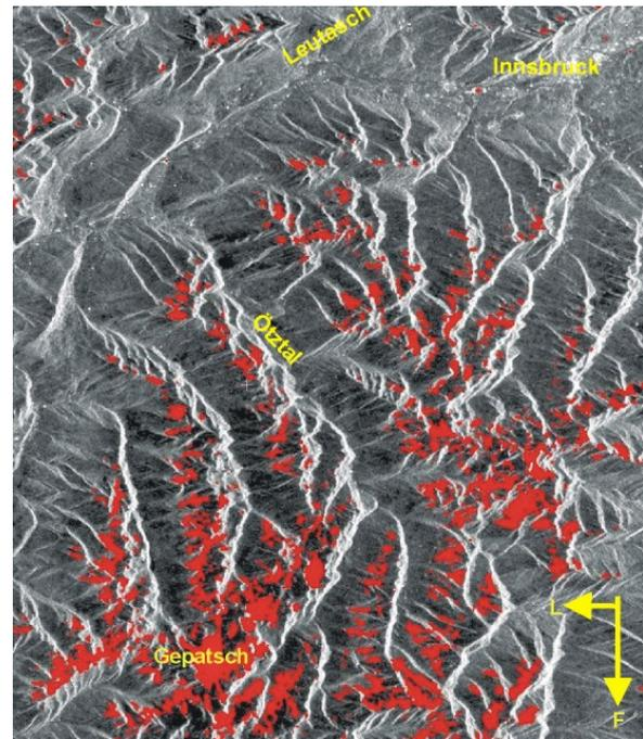
Fig 11: Change of wet snow area from 10 May to 14 June 2003 (red), from ASAR WSM data, VV polarisation. The snow map is overlaid to the amplitude image in ground range geometry.
