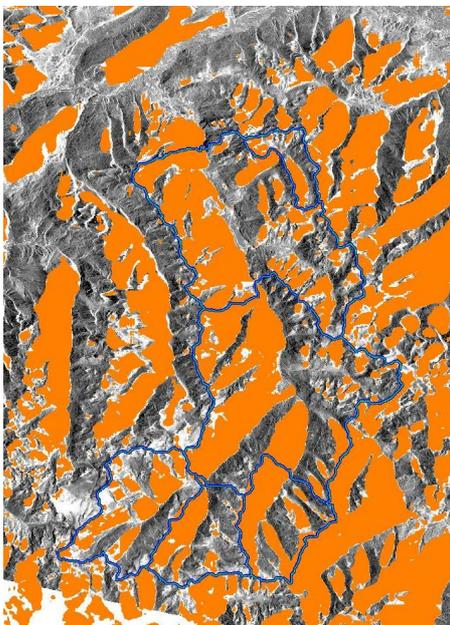
Fig. 7: Geocoded multitemporal amplitude image of ASAR swath IS-2, track 437. Layover areas are shown in orange, the blue line outlines the Ötztal basin.
