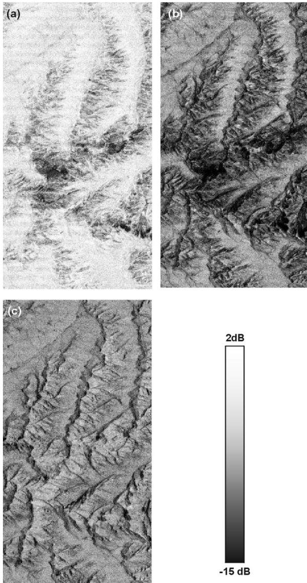
Fig. 9: Multitemporal ratio images of wet snow (10 May) versus dry snow reference (21 Dec.) and single track ratio). Multitemporal approach: (a) 10 May 2003 (AP, VV) versus 21 Dec 2002 (IM, VV), (b) 10 May 2003 (AP, VH) versus 21 Dec 2002, (IM, VV). Single track approach (c) 10 May 2003 (AP): VH versus VV.
