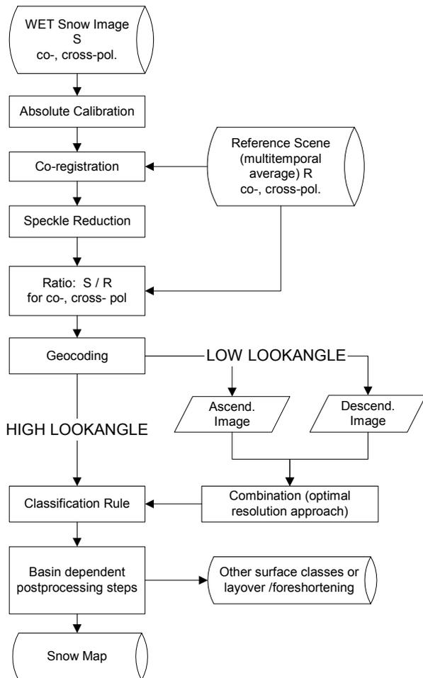
Fig. 5: Processing steps of SAR based wet snow mapping procedure (using ASAR Image mode and/or Alternating Polarisation Mode Products).
