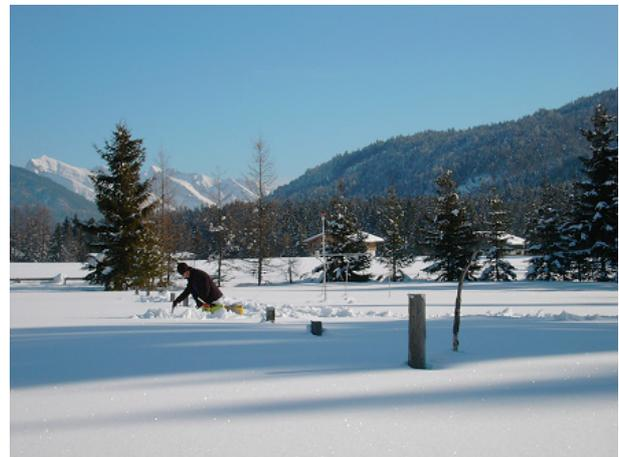
Fig. 3: Test site Leutasch, 1100 m, with automatic meteorological station providing measuring air temperature, wind, solar radiation, snow temperature at 3 levels, and soil temperature.
