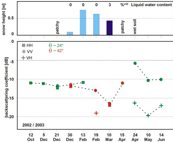
Fig. 4: Backscatter signatures (multi-looked) of meadow with and without snow at the Leutasch test site (lower diagram). The upper graph shows corresponding measurements of snow height and liquid water content.
